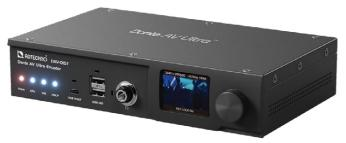
for video preview, audio level meters, and Dante settings adjustments, these devices ensure seamless integration and precise control. With PoE+ support, advanced signal management, and compatibility with Dante Controller, the DAV-01 series is ideal for professional AV applications, including stadiums, boardrooms, and high-end conference environments.
