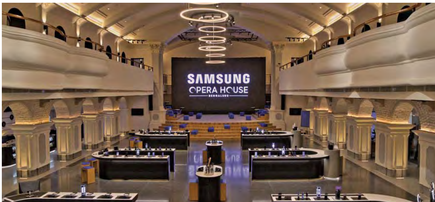
Samsung's largest mobile experience centre in the world in Bangalore includes an indoor and an outdoor video wall. The indoor videowall (9.6m x 5.4 m) deployed by Hewshott, has a 2.5 mm pixel pitch and 4K resolution.
