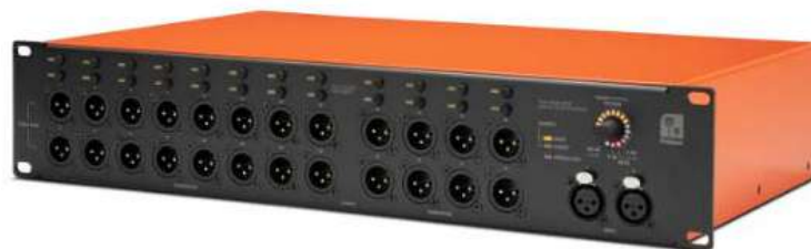
Grand Audition MKII, a 19" loudspeaker switching system
