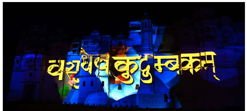
Twelve Barco UDX-4K40 projectors used alongside Dataton's Watchout software resulted in a breathtaking 3D projection mapping at the venue
