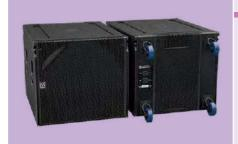
The SXCF118 is a compact, high-performance cardioid subwoofer. The flown version of the SXC118 is the ideal partner for flown WPS arrays — combining maximum low-frequency output with pattern control. It features an 18" (460mm) forward-facing driver and a 14" (356mm) rear-facing driver, each driven independently by separate amplifier channels and DSP. Each driver has its chamber with an optimised bass reflex port.
