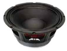
cies ideal for live sound and recorded music venues. The transducer uses high energy ferrite based magnetics to achieve a very high acoustic output to weight ratio with a die-cast aluminium design that insures a very high degree of structural integrity. The E10-300A has been optimized for use in two way or three-way sound reinforcement systems and has an operating range of 50Hz to 5000Hz.
